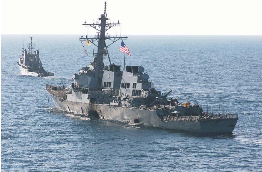
Figure 16-5.—Three-quarter aerial bow photograph of bomb-damaged USS Cole (DDG 67) being towed into open sea by the USNS Catawba (T-ATF-168).
