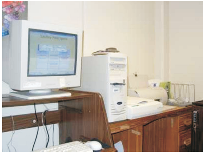
Figure 8-1.—The components of a typical desktop publishing system: personal computer, laser printer, scanner, mouse and software.
